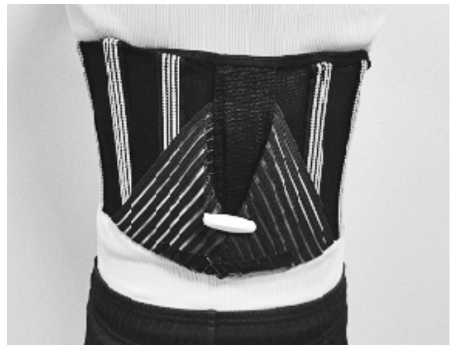
Fig. 2 The accelerometers lie over the middle of the lower back in a semi-elastic belt fastened around the subject's waist.
