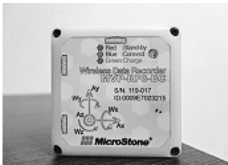
Fig. 1 Accelerations in a \pm 60\text{m/sec}^2 range were measured using a lightweight (60g) tri-axial accelerometer (MicroStone Ltd., Japan)
